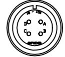
DETAIL "A" VIEWED FROM WIRE SIDE OF CONNECTOR AMPHENOL SOCKET INSERT MS18-10S (MCM495)
