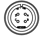
DETAIL "B" VIEWED FROM WIRE SIDE OF CONNECTOR AMPHENOL SOCKET INSERT MS18-10S (MCM495)
