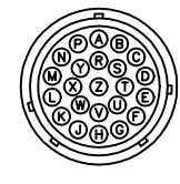
DETAIL "C" BURNDY PLUG UTG618-23SN (ECK135) VIEWED FROM WIRE SIDE OF CONNECTOR
