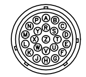
DETAIL "C" BURNDY PLUG UTG618-23SN (ECK135) VIEWED FROM WIRE SIDE OF CONNECTOR
