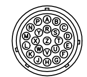
DETAIL "B" BURNDY PLUG UTG618-23SN (ECK135) VIEWED FROM WIRE SIDE OF CONNECTOR
