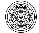
DETAIL "B" BURNDY PLUG UTG618-23SN (ECK135) VIEWED FROM WIRE SIDE OF CONNECTOR
