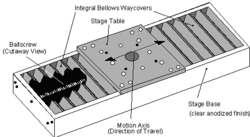
Figure 1-2: ATS150 with Cutaway View of Ballscrew
