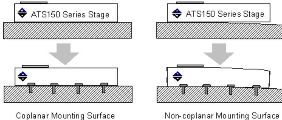
Figure 2-1: Results of Coplanar Versus Non-Coplanar Mounting
